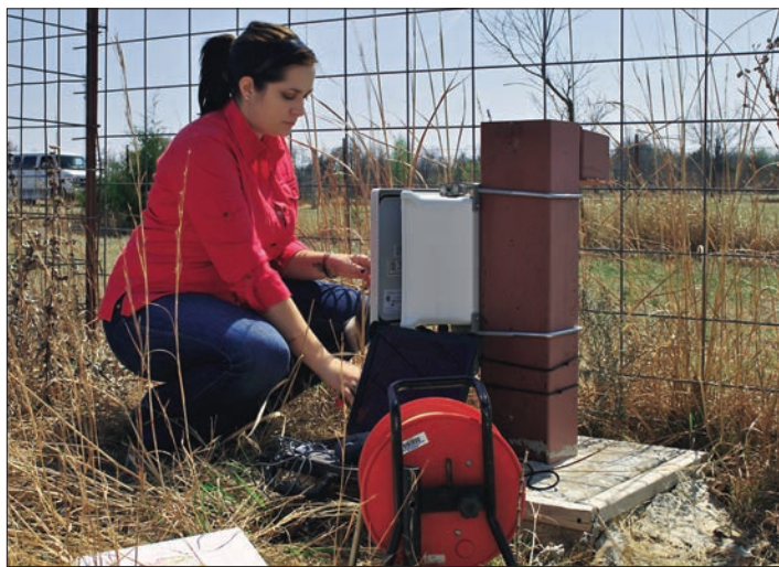
OWRB geologist Jessica Magers measures the groundwater level at the Spencer Mesonet site. The well was installed at the site to collect data for the Garber-Wellington Management Study. This is one of six Mesonet sites statewide with a groundwater observation well.
