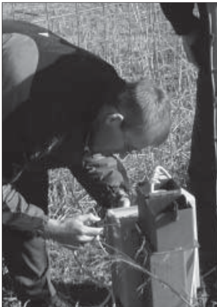
Water Board Geologist Greg Gromadzki checks the automated data logger at the El Reno Mesonet site's observation well.
