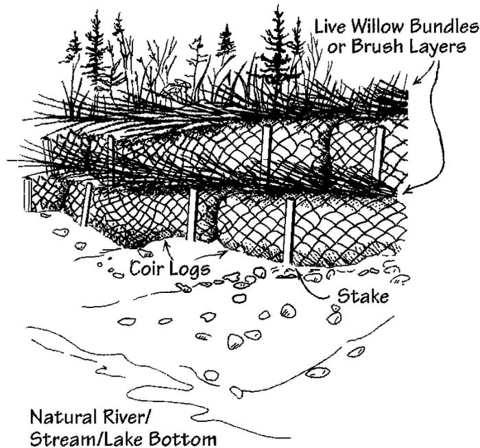
**Figure 2.11: Drawing showing coir geotextile rolls (CGRs) with live willow cuttings inserted between and above the CGRs.**
