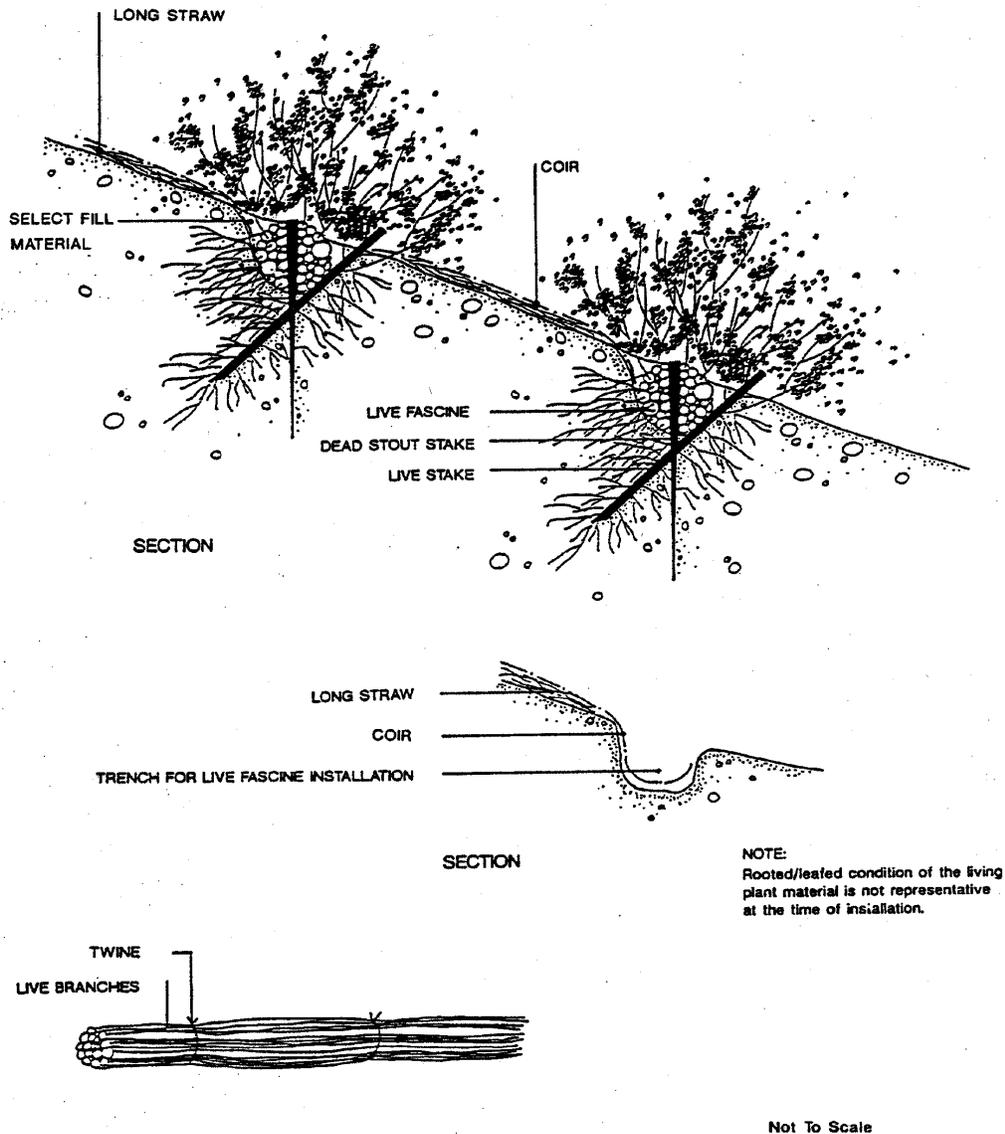
Figure 2.19: Drawing of fascines with erosion control fabric (coir) in between
