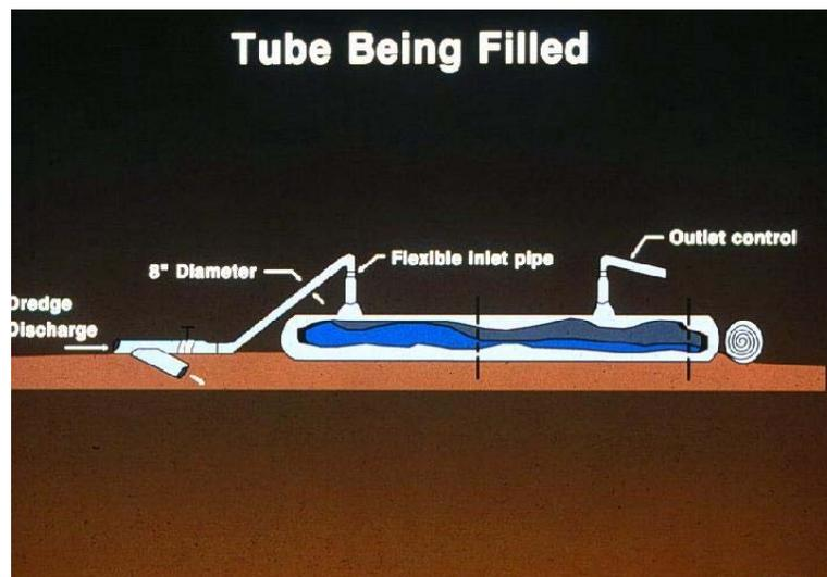
Figure 2.25: Drawing illustrating a geotube being filled from a dredge pipe.
