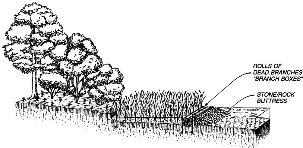
**Figure 2.16: Schematic of branchbox breakwater with emergent aquatic vegetation (EAV) shoreward of it.**
