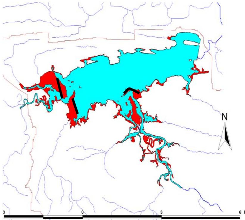
**Figure 2.23: Proposed placement of breakwaters to reduce wave action and suspended solids in Lake Wister.**
