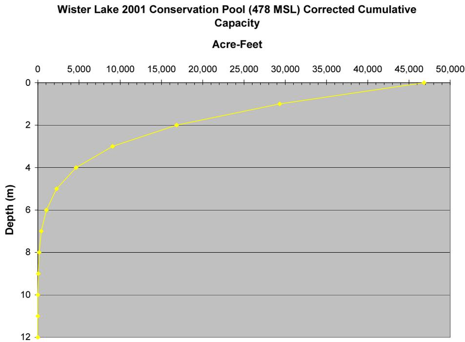
**Figure 4.5: Wister Lake 2001 Corrected Cumulative Capacity Curve.**
