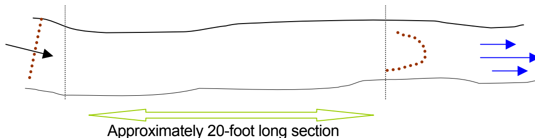
Figure 2. General setup for measuring discharge using floats
