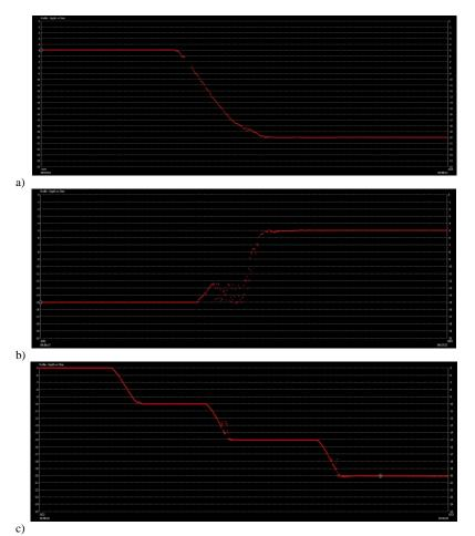
Figure 4: Digital Echogram of Bar-checks for All Lakes Surveyed a) Brushy Creek Lake 11/29/17 b) Greenleaf Lake 12/06/17 c) Shell Lake 03/28/18
