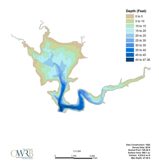
Figure D- 2: Shell Lake Contour Map with 5 ft Intervals.
