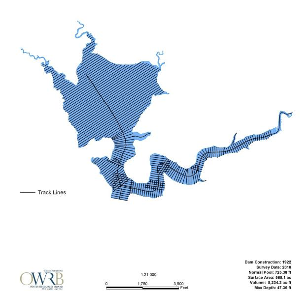
Figure D-1: Shell Lake Survey Track Lines Map.
