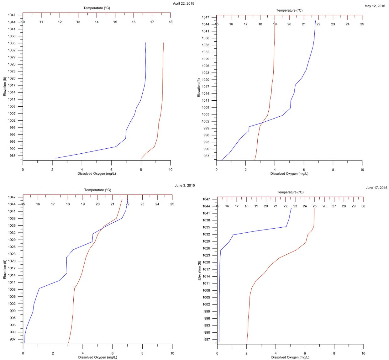
**Figure 7. Temperature (red) Dissolved Oxygen (blue) Vertical Profiles. Site 1: April 24, 2015 – June 17, 2015.**
