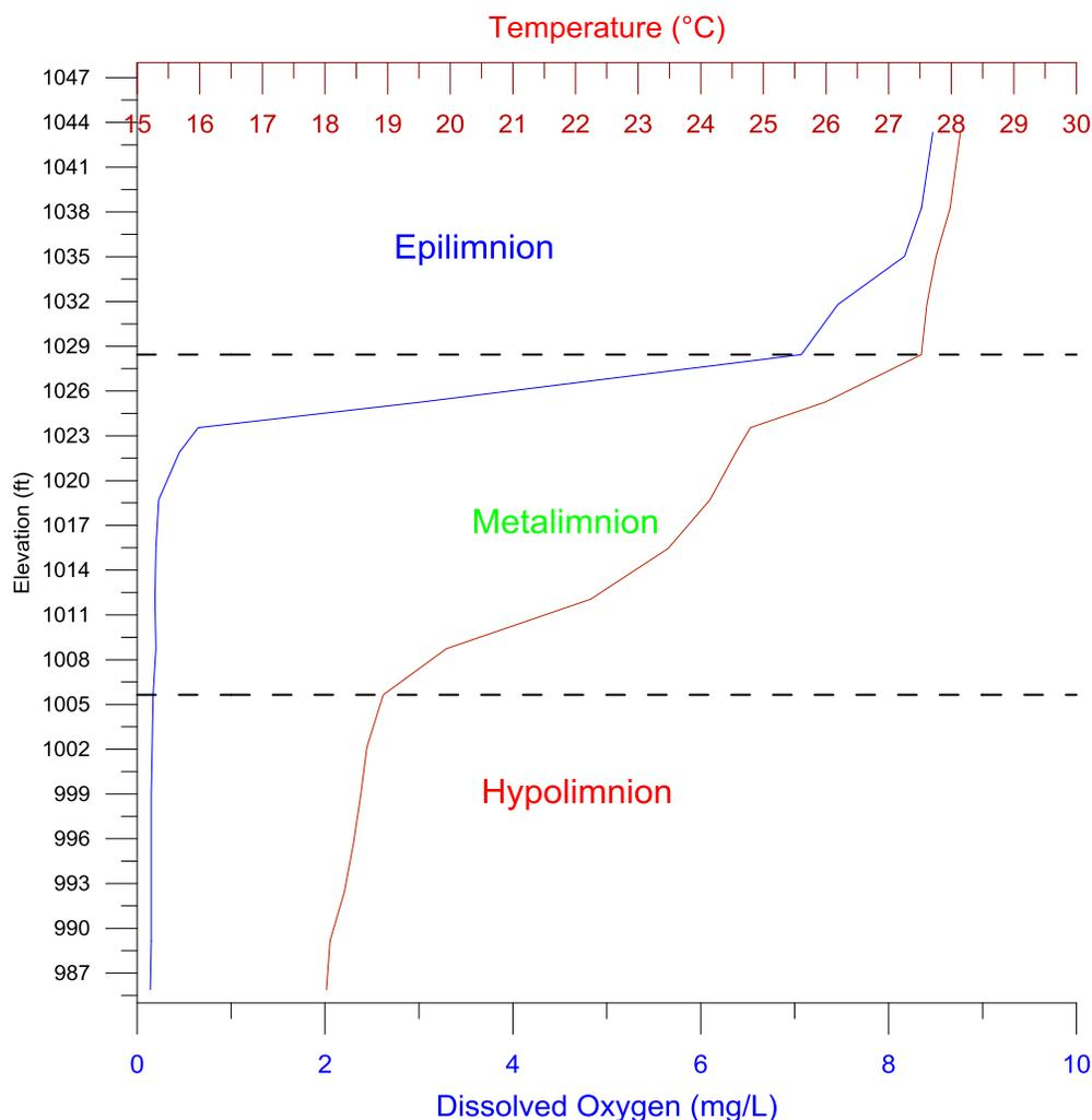
**Figure 6. A Typical Temperature and Dissolved Oxygen Vertical Profile for Lake Thunderbird (July 1<sup>st</sup>, 2015) Approximate Boundaries Between the Epilimnion, Metalimnion and Hypolimnion are Marked with Dashed Lines.**
