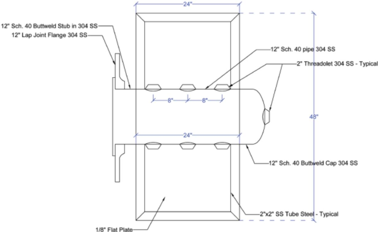
Figure 36. Schematic of the Modified Nozzle
