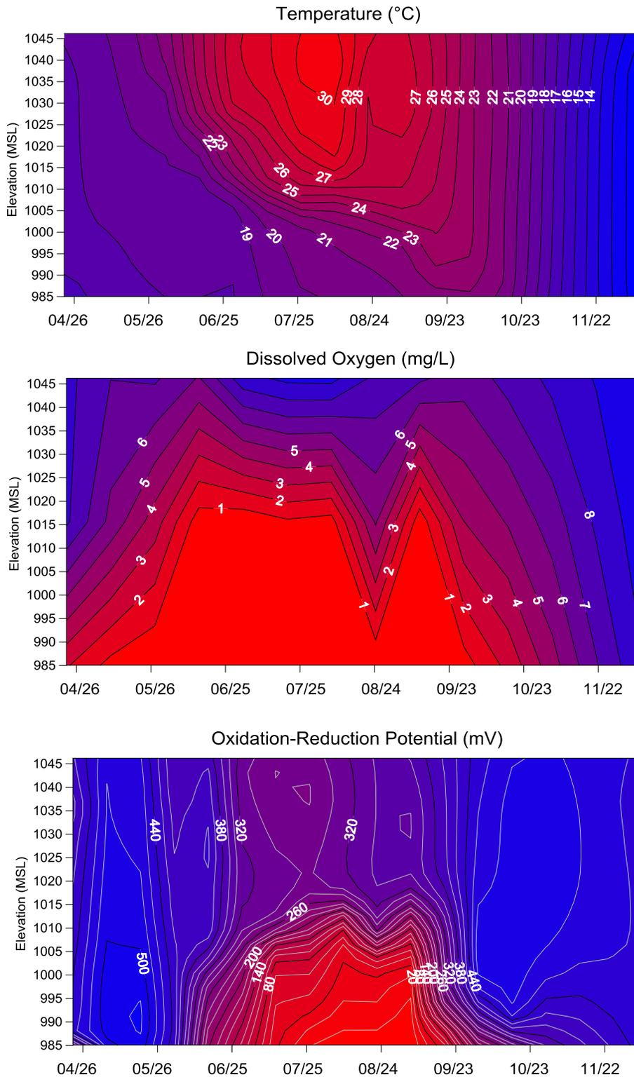
**Figure 37. Temperature, Dissolved Oxygen and Oxidation-reduction Potential (ORP) by Elevation for 2015 Site 1 Lake Thunderbird; Highlighting the Temporal Disparity Between Onset of Stratification (Temperature), Anoxia (Dissolved Oxygen) and Reducing Conditions (ORP).**
