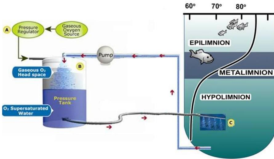
**Figure 34. Conceptual Illustration of the SDOX System at Lake Thunderbird**
