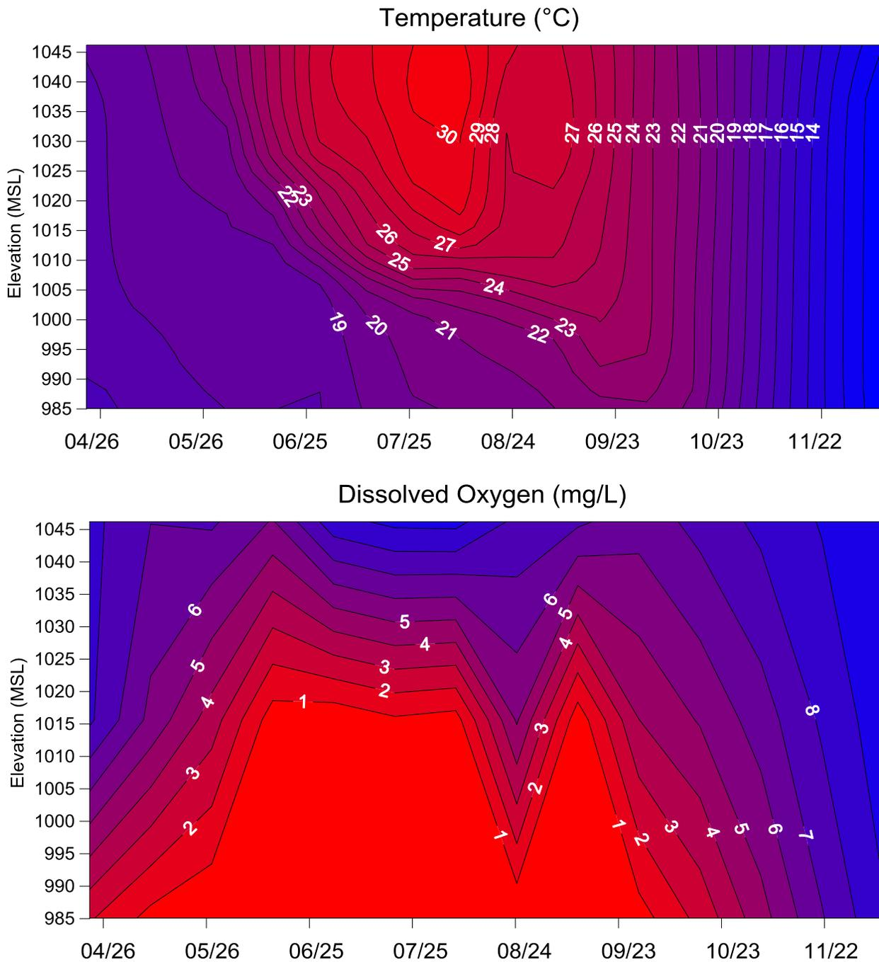
**Figure 10. Isopleths of Temperature (°C) and Dissolved Oxygen (mg/L) by Depth (m) Lake Thunderbird 2015.**
