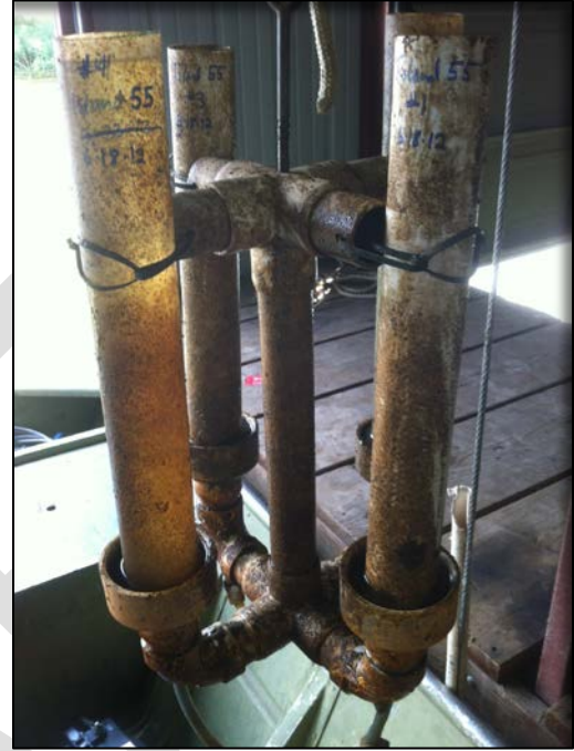
Figure 10 Sediment trap retrieved from under the floating wetlands.
