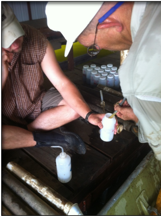
Figure 11 Transferring collected sediment from the trap into the sample bottle.
