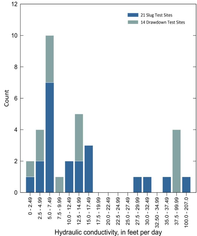
**Figure 26.** Histogram showing the hydraulic conductivity distribution of slug tests and drawdown data.
