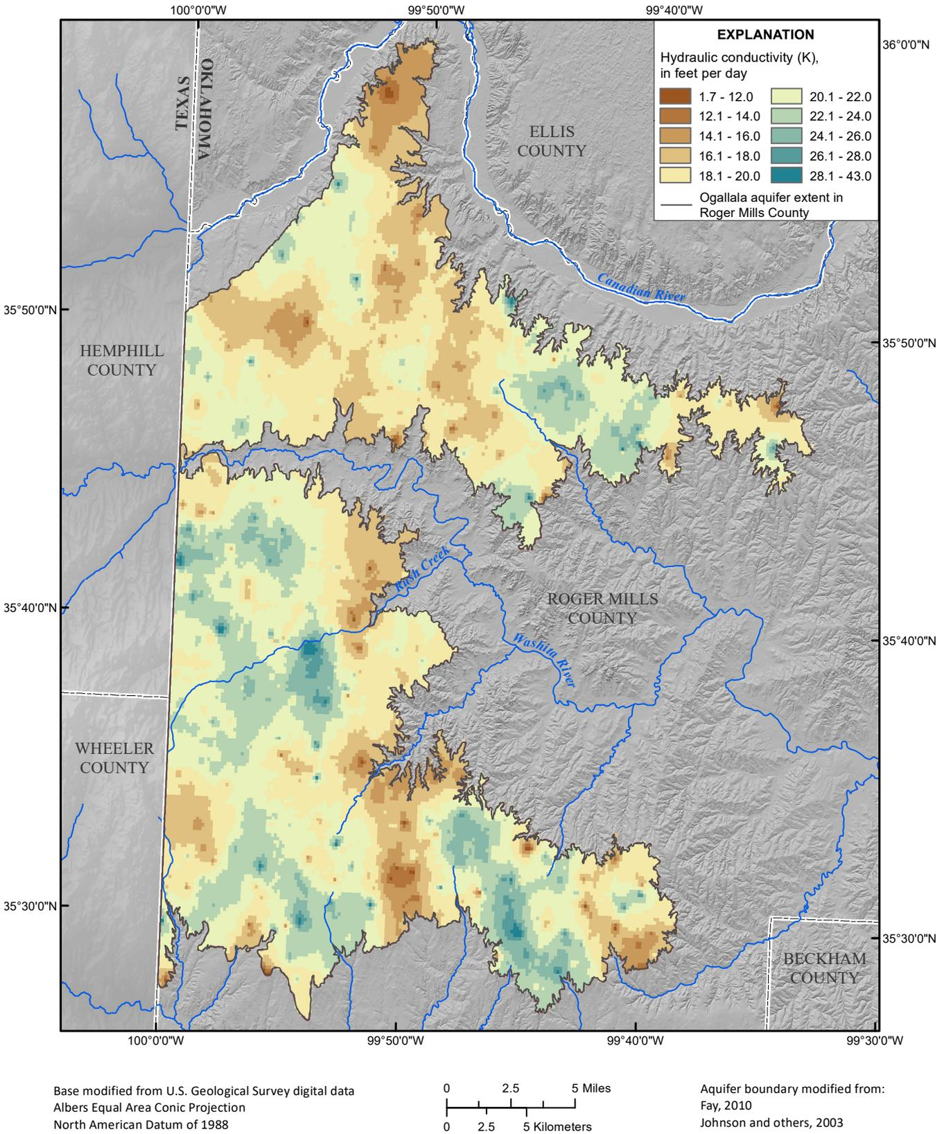
**Figure 29.** Estimated horizontal hydraulic conductivity using percent-coarse analysis.
