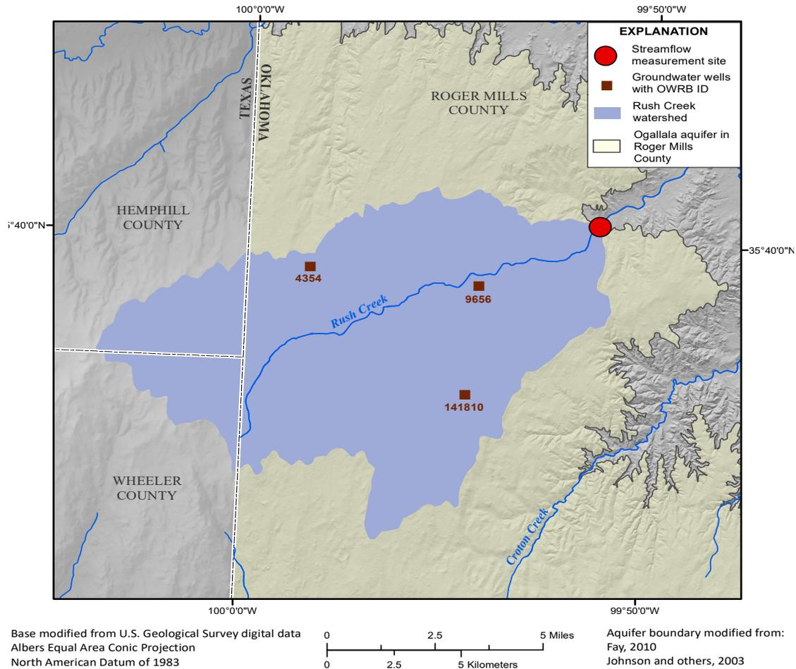
**Figure 30.** Groundwater wells and streamflow measurement sites in the Rush Creek watershed used for the regional method to determine specific yield.
