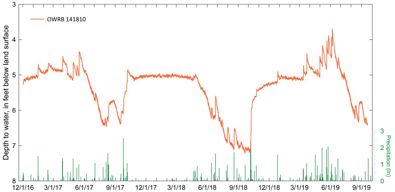
**Figure 11.** Water levels from OWRB continuous water-level well and precipitation data from the Cheyenne Mesonet station showing short-term responses to precipitation and seasonal patterns (see Figure 1 for location).
