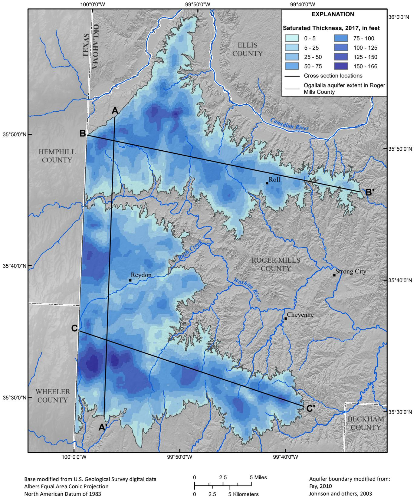
**Figure 18.** Saturated thickness (2017) and cross-section locations in the Ogallala aquifer in Roger Mills County.
