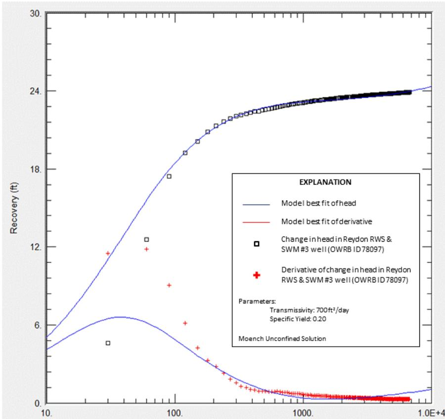
**Figure 27.** Recovery draw-down curve and derivative with best-fit Moench method for the Roger Mills Rural Water, Sewer & Solid Waste Management #3 single-well aquifer test at site 78097.
