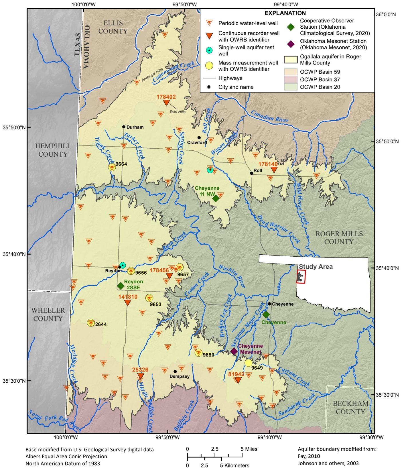
**Figure 1.** The Ogallala aquifer in Roger Mills County and study area, with locations of continuous water-level recorder wells, water levels collected by the OWRB, weather stations, and OCWP basins.
