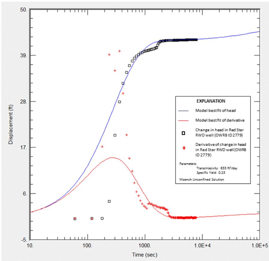
**Figure 28.** Drawdown curve and derivative with best-fit Moench method for the Red Star Rural Water District single-well aquifer test at site 2779.
