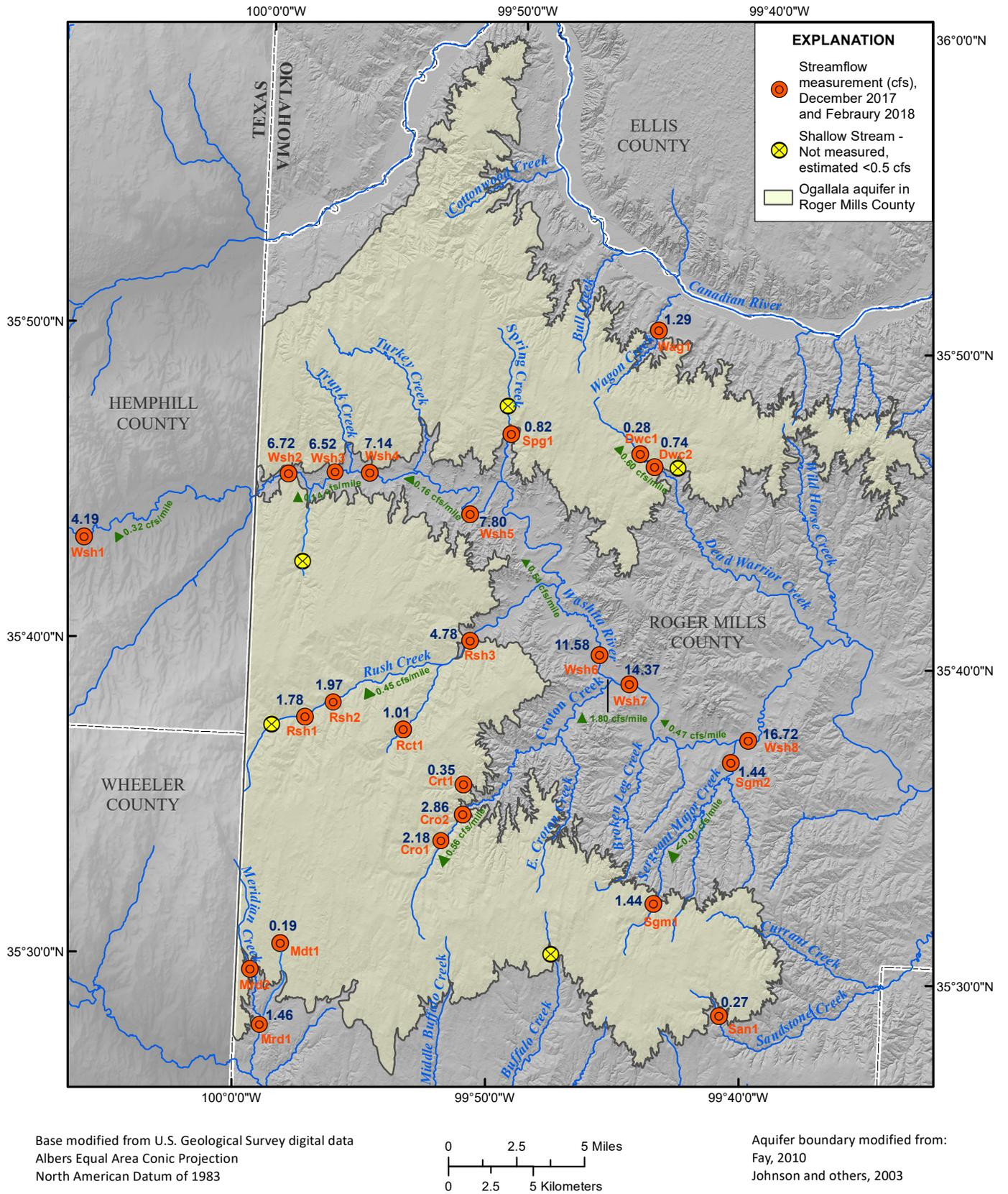
**Figure 8.** Streamflow measurements in cubic feet per second and locations, December 2017 and February 2018.
