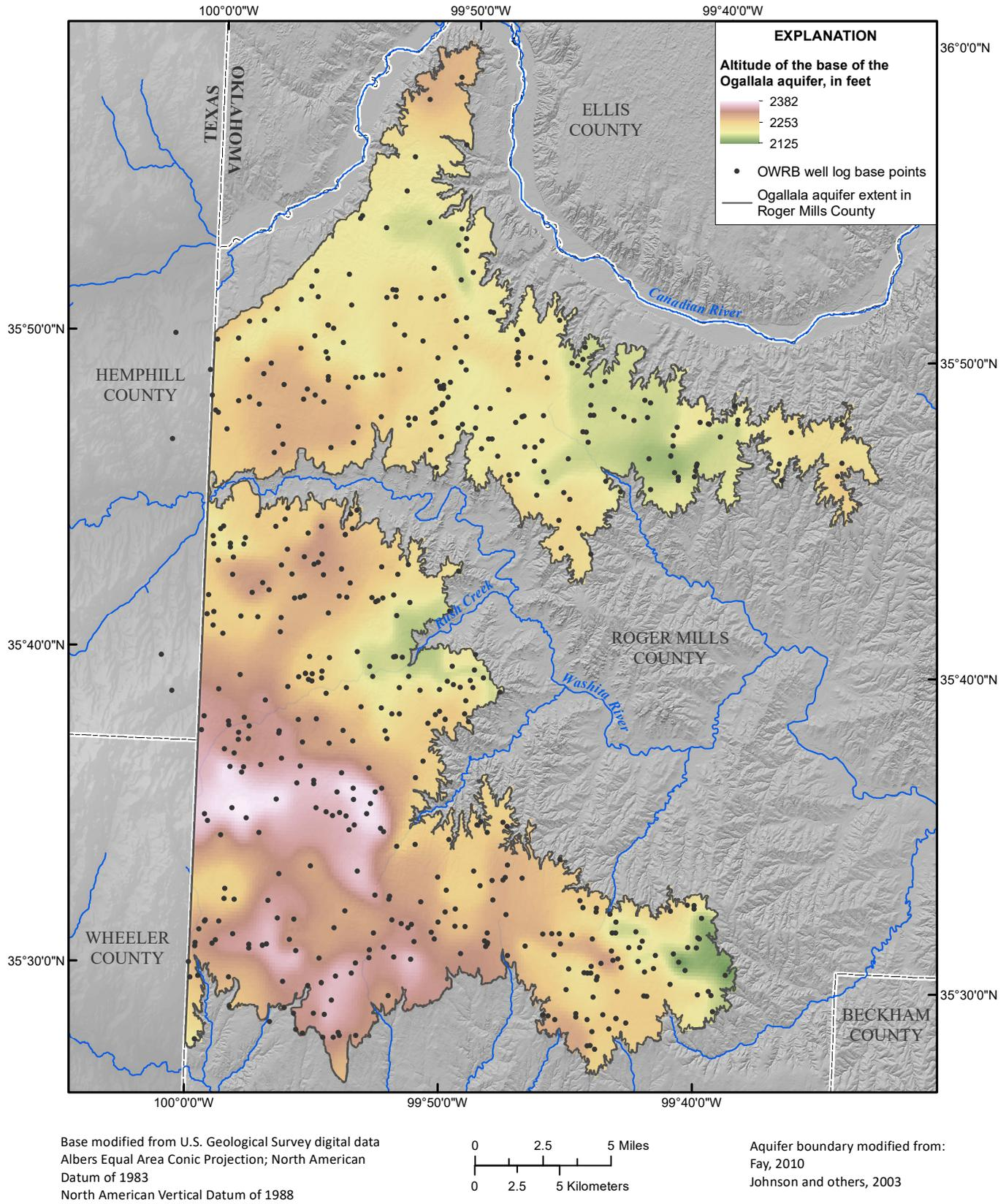
**Figure 17.** Elevation of the base of the Ogallala aquifer in Roger Mills County derived using lithologic logs.
