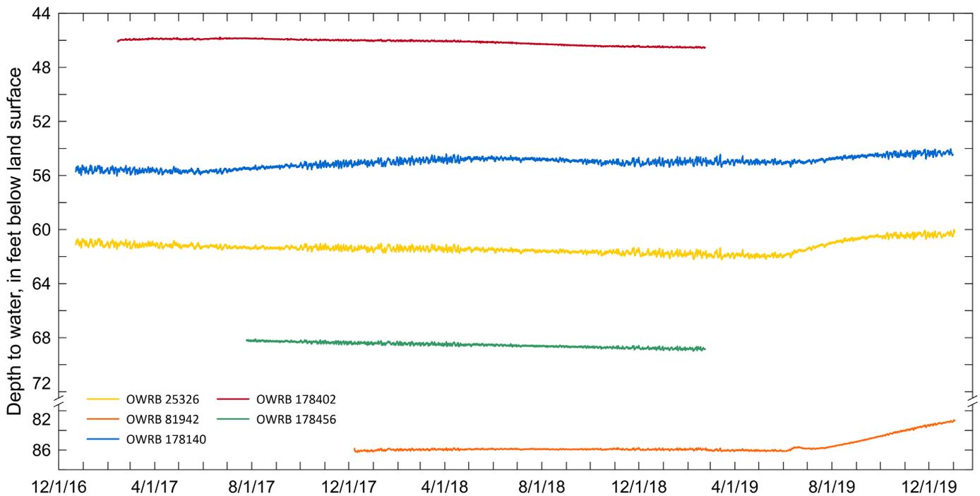
**Figure 12.** Water levels from OWRB continuous water-level recorder wells (see Figure 1 for locations).
