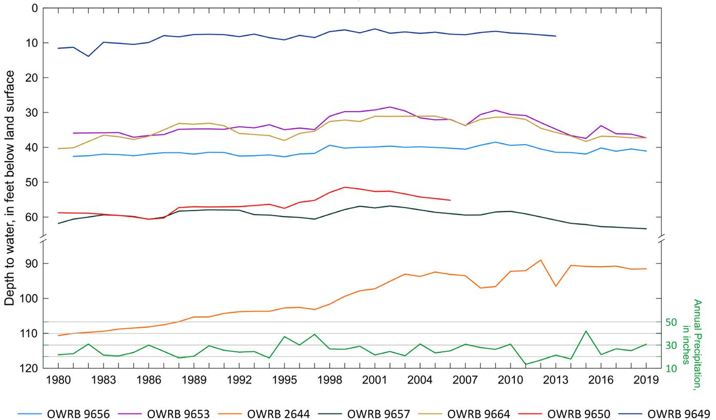
**Figure 10.** Water levels from OWRB Mass Measurement Program wells showing long-term responses (see Figure 1 for locations).
