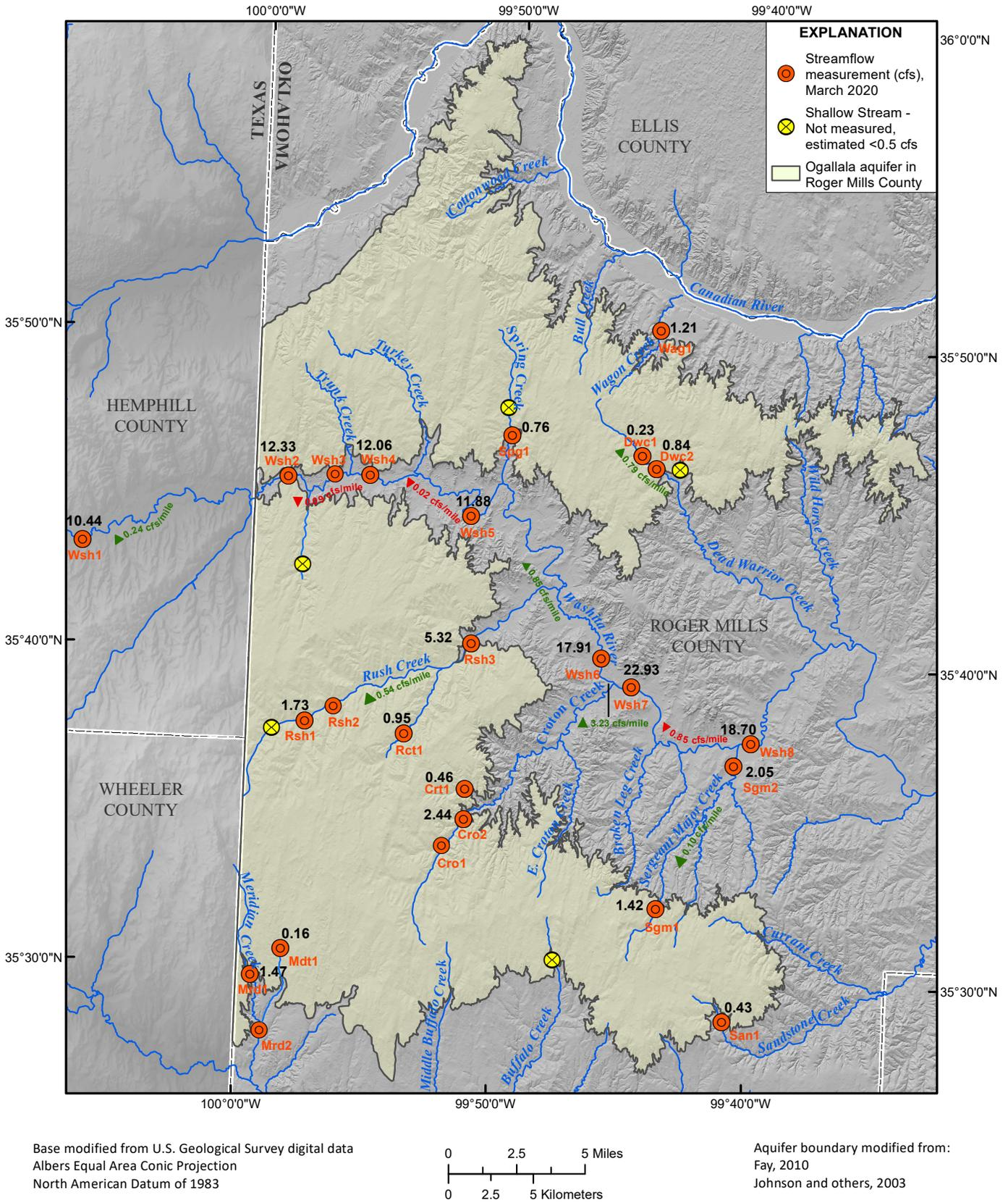
Figure 9. Streamflow measurements in cubic feet per second and locations, March 2020.
