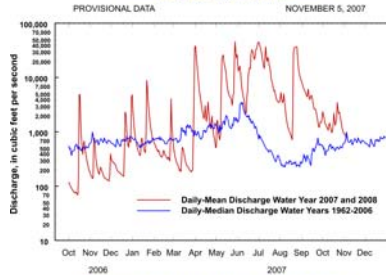
Comparison of daily discharges for water year 2007 and 2008 and period of record Data from U.S. Geological Survey
