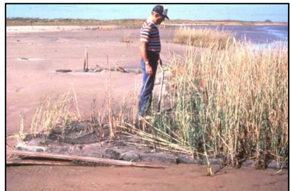
Figure 20. Same erosion control mat to left after 3 years
