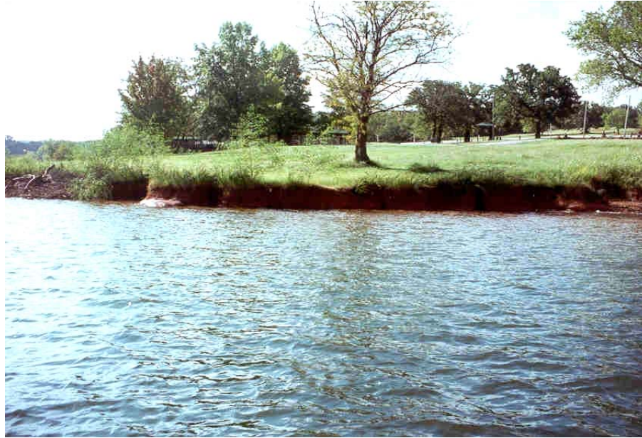
Figure 7. Category 5 erosion; about a 4-ft escarpment without a toe or bench at Clear Bay Cafe area.
