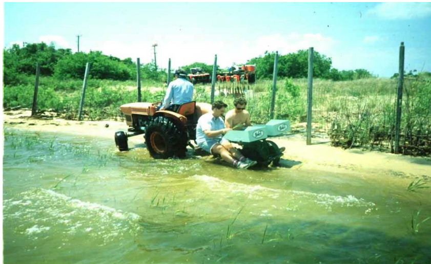
Figure 9. Planting emergent aquatic plants using a tobacco planter and tractor
