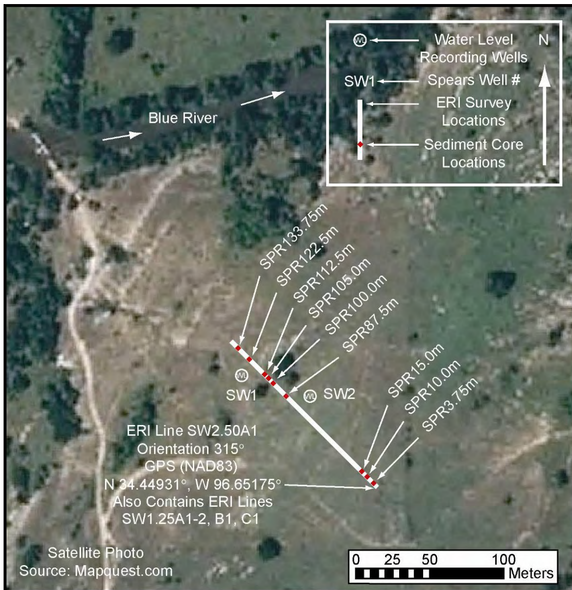
Figure A1.8B. Spears Ranch site map with surface electrical resistivity and direct push locations and well locations (from Sample, 2008). Aerial photo courtesy of Mapquest.
