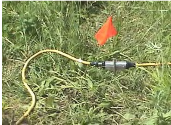
Figure 2. Surface electrodes used to collect resistivity data.
