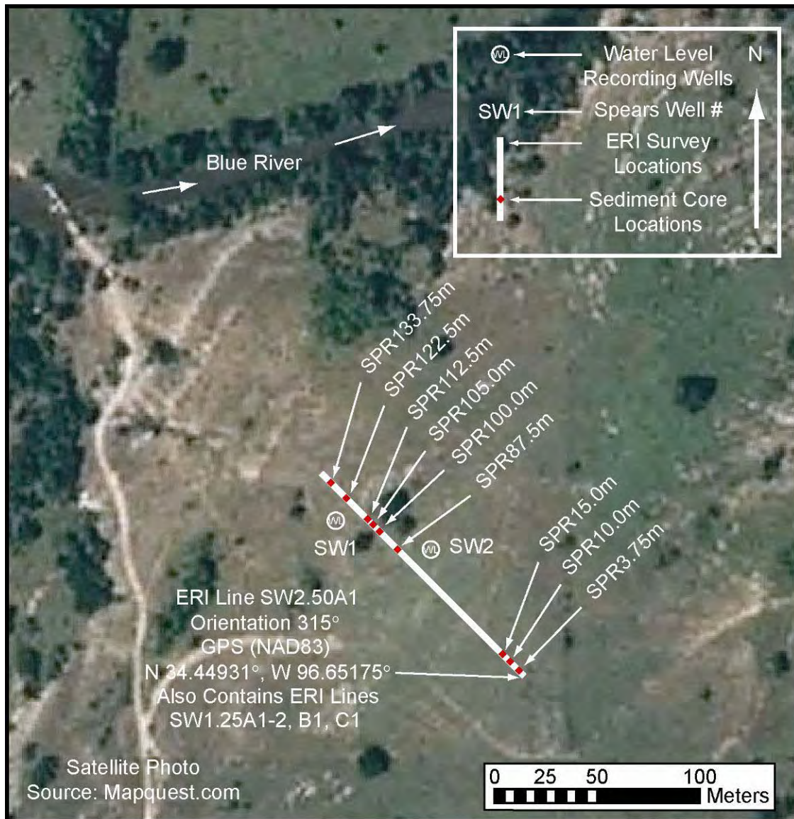
Figure 15. Spears Ranch site map with surface electrical resistivity and direct push locations and well locations (from Sample, 2008). Aerial photo courtesy of Mapquest.
