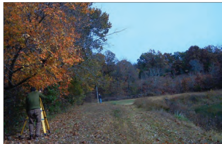
OWRB dam safety staff measure the elevation of a dam in Adair County to determine its hazard classification.
