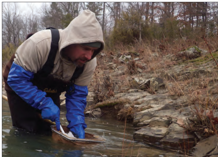
OWRB biologist Josh Bailey collects winter macroinvertebrate (aquatic insect) samples from the Mountain Fork River near Smithville in southeast Oklahoma. An analysis of these samples provides critical information about the water quality conditions of the stream segment.
