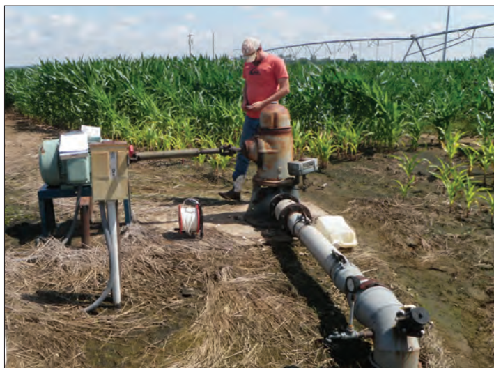
OWRB groundwater specialist Kevin Kilhoffer measures and samples an irrigation well at a GMAP site in the Arkansas River alluvial aquifer.
