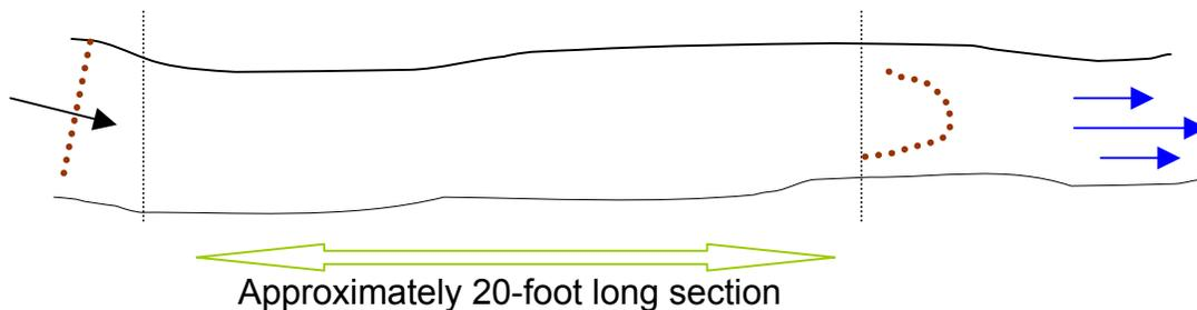
Figure 2. General setup for measuring discharge using floats
